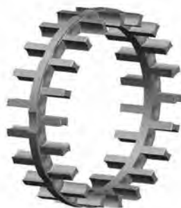
Fig. 4. One-piece finger-type cage.
