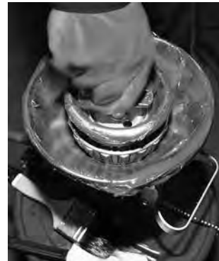
Fig. 15. Mechanical grease packer.
