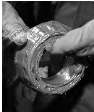
Fig. 14. Grease can easily be packed by hand.
